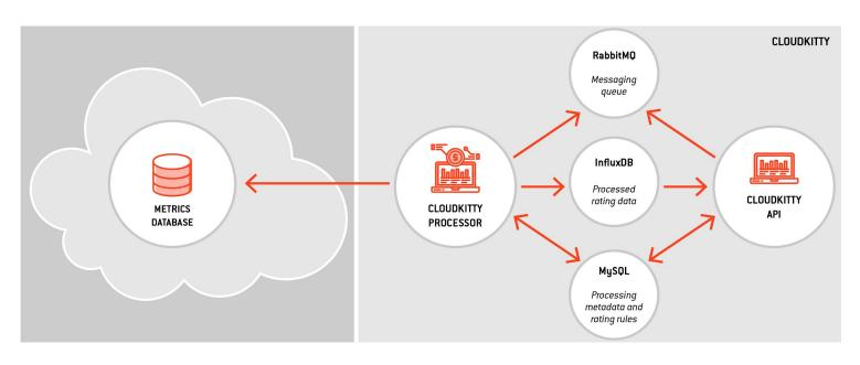
All CloudKitty components in a standard deployment
